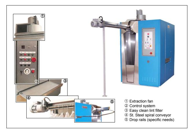
BMM Weston Tunnel Finishers are a modular range of ruggedly constructed, simple to operate, compact, hot air / steam finishing tunnels.
